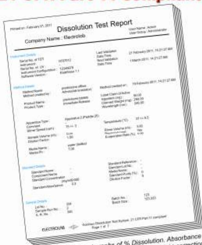
Choice for Table and graphs of % Dissolution, Absorbance and concentration with/without volume and weight correction. Report includes rpm, temperature validation table, statistical functions as min, max., mean, standard deviation and standard deviation. Consolidated report of all stages
